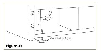
Check the levelness after each adjustment and repeat the previous steps until the unit is level. Go on to 9 Install the Unit.
